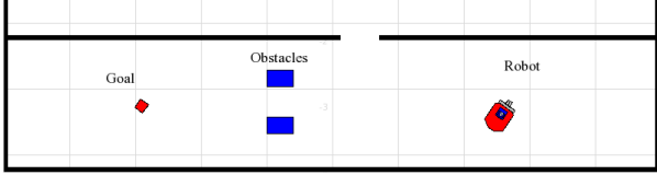
Fig. 1. The scenario in the initial state. The robot (right-hand side) is expected to surpass the obstacles in the middle and reach and grip the goal object (left-hand side).
