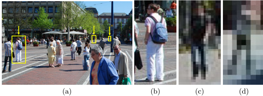
Fig. 2. A standard image of an urban scene. (a) Three pedestrians of different size are marked by the yellow arrows and boxes. (b-d) Close-ups of the marked objects using nearest-neighbor interpolation for resizing. Even though humans can recognize the objects at all three scales, it is obvious that the bigger pedestrian in (b) is easier to detect than the ones in (c) or (d).
